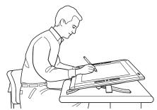
Adjust the display stand to a lower position as needed to emulate an easel, animator's table, or drafting table.
