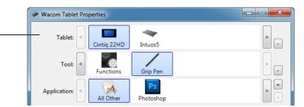
To add a new pen display or tablet, connect it to your computer. The system will automatically find the pen display or tablet and initialize it. An icon for the pen display or tablet will then appear in the control panel.
