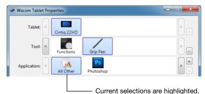
The TOOL list displays icons for the pen display FUNCTIONS and for the different tools that have been used on the pen display.
